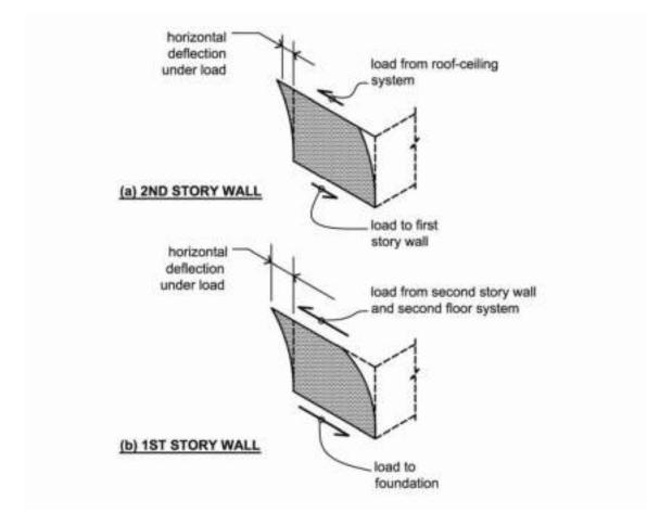
Figure 2-4 Loading and deflection of bracing wall systems.
