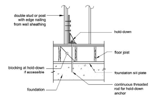
Figure 9-7 Weak- and soft-story bracing.
