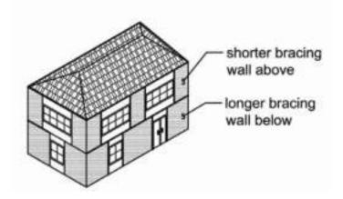
Figure 2-8 Ideal building configuration for earthquake resistance.
