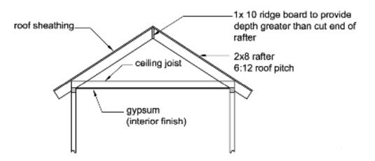
Figure 6-1 Typical light-frame roof-ceiling system.
