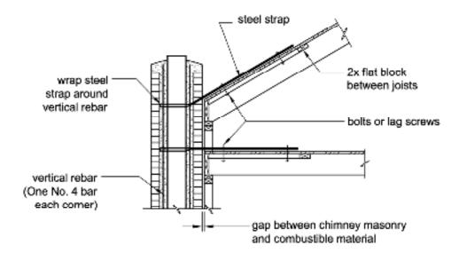
Figure 7-4 Chimney section showing earthquake anchorage.
