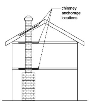
Figure 7-3 Locations for earthquake anchorage of masonry chimney at exterior house wall.
