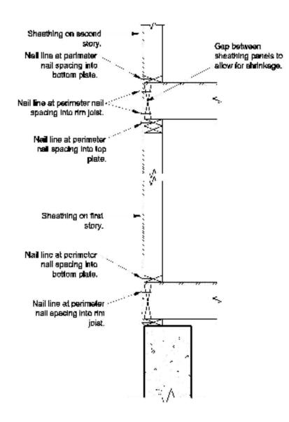
Figure 5-10 Sheathing detail for extending the sheathing over the band joist.
