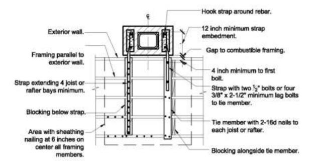
Figure 7-5 Anchorage detail for framing parallel to exterior wall.
