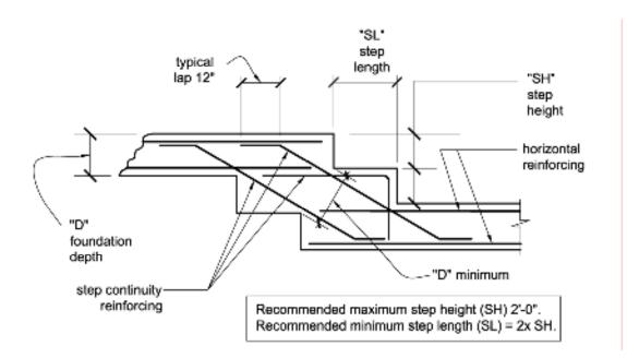
Figure 3-11 Above-code stepped foundation reinforcing detail.
