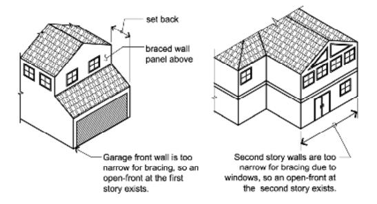
Figure 9-8 Common open-front occurrences in one- and two-family detached houses.
