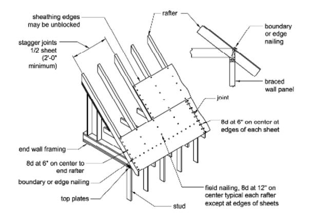
not staggered. Typical wood structural panel roof sheathing installation using staggered joints is illustrated in Figure 6-5.
