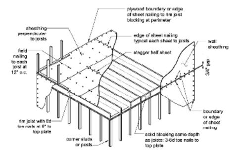
Figure 4-1 An unblocked floor diaphragm.
