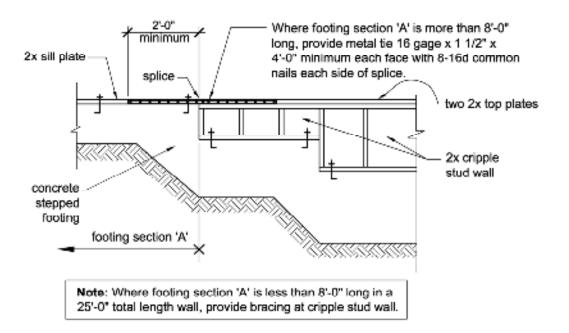
Figure 2-17 Detailing required for stepped foundation walls (ICC, 2003).
