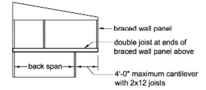
Figure 4-3 Cantilevered floor restrictions.
