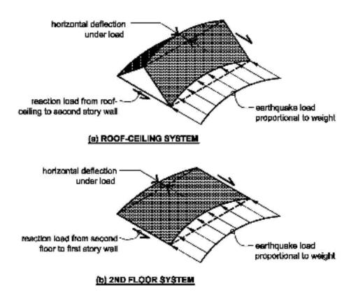
Figure 2-3 Loading and deflection of roof-ceiling and floor systems.
