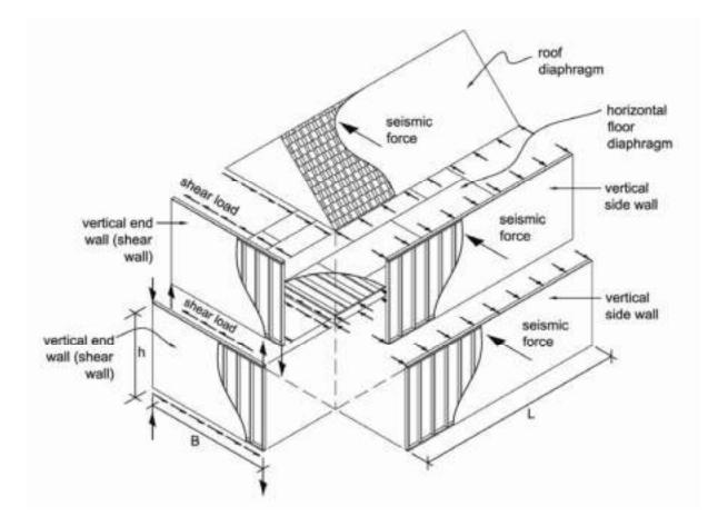
Figure 2-5 Load transfer between components in a building.
