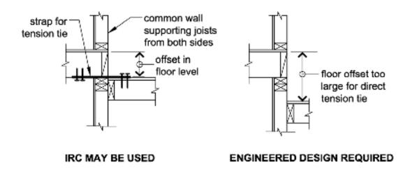
Figure 9-12 Split-level ties for floor framing.
