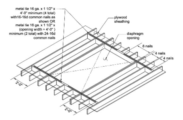
Figure 4-11 Reinforcing straps at large diaphragm openings.
