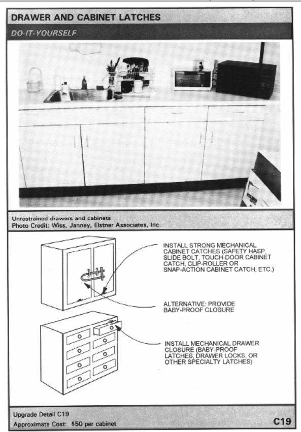
Figure 8-3a Reproduction of FEMA 74 suggestions for securing drawer and cabinet latches.
