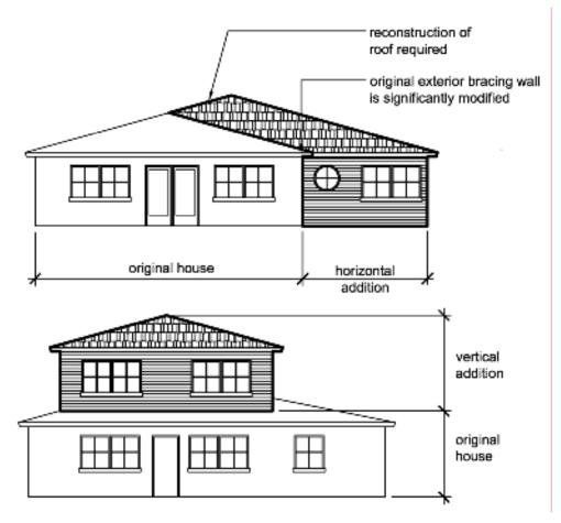
Figure 9-2 Horizontal addition (above) and vertical addition (below).
