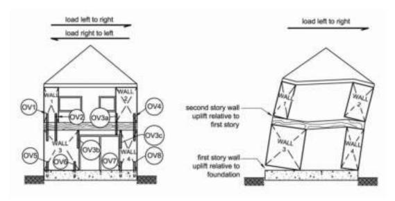
Figure 2-7 Overturning load path connections and deformations.
