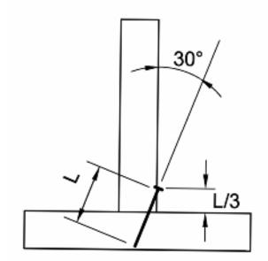
Figure 4-8. Toe nail configuration requirements.
