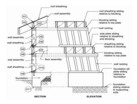
Figure 2-6 Horizontal load path connections and deformations.
