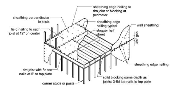
Figure 4-9 Blocked diaphragm configuration.
