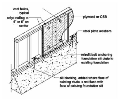
Figure 9-6 Cripple wall bracing.
