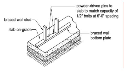
Figure 3-14 Interior braced wall on slab-on-grade.
