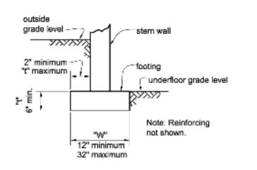
Figure 3-9 Inverted -T footing dimensions.
