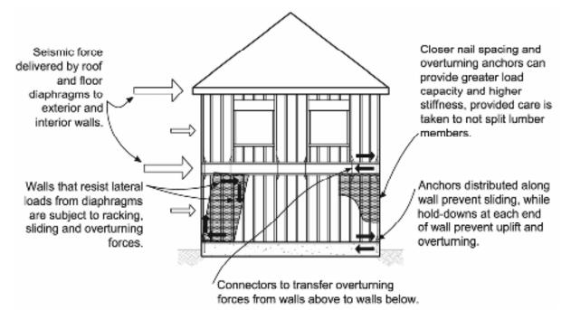
Figure 5-3 Wall action for resisting lateral loads
