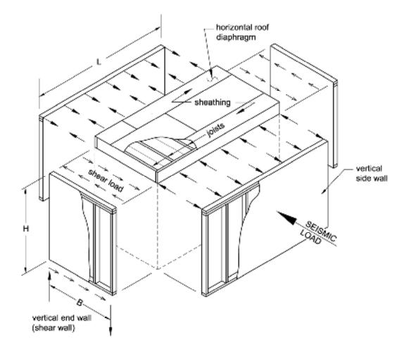
Figure 5-2 Exploded view of house illustrating load paths.
