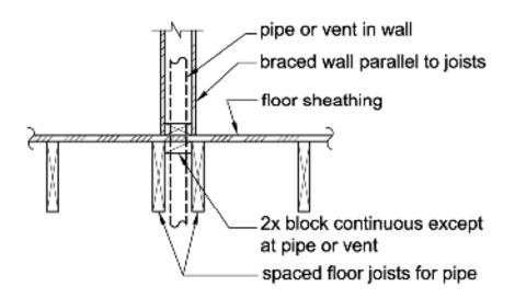
Figure 4-7 Blocking for floor joists spaced apart for piping in floor.
