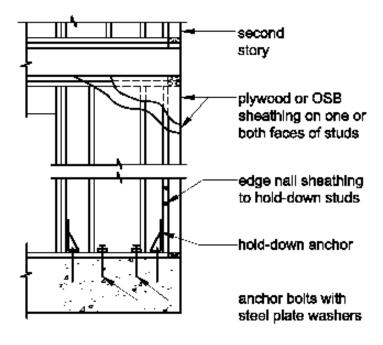
Figure 9-9 Detailing of narrow bracing wall piers at open fronts.
