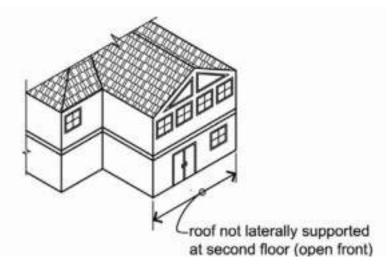
Figure 2-9 Irregular building configuration with open front (no second-story bracing walls supporting roof on right-hand portion).
