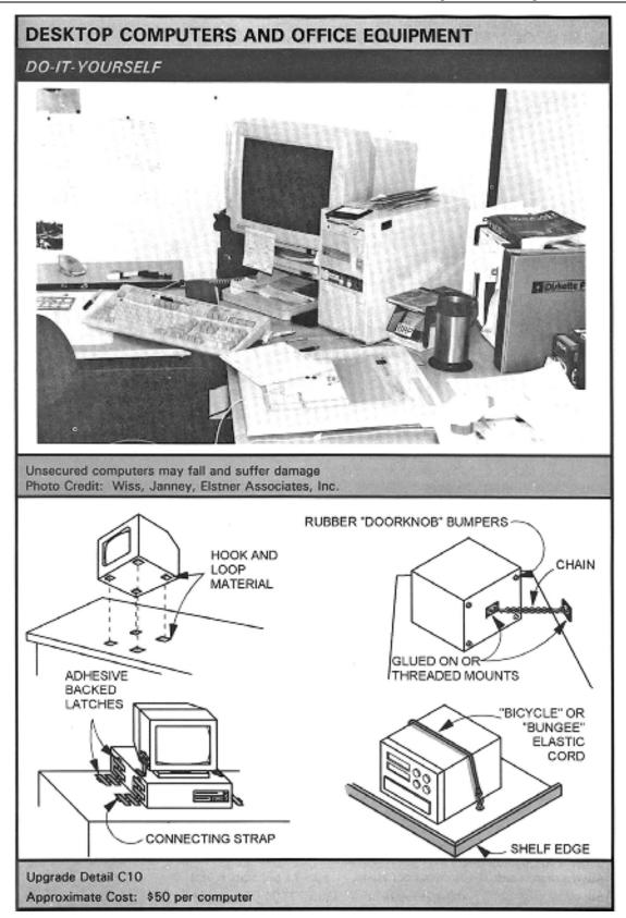
Figure 8-3c Reproduction of FEMA 74 suggestions for securing desktop computers and office equipment.
