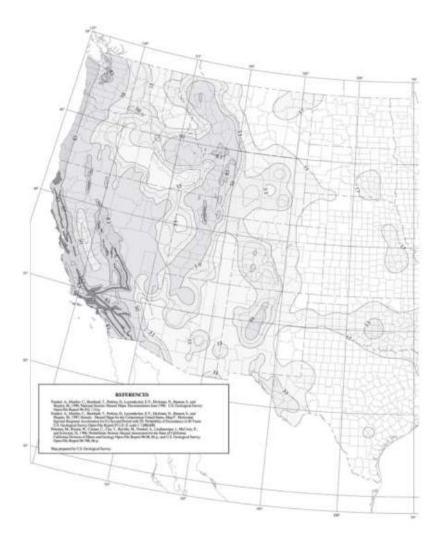
Figure 1-1 Seismic Design Categories – Site Class D.
