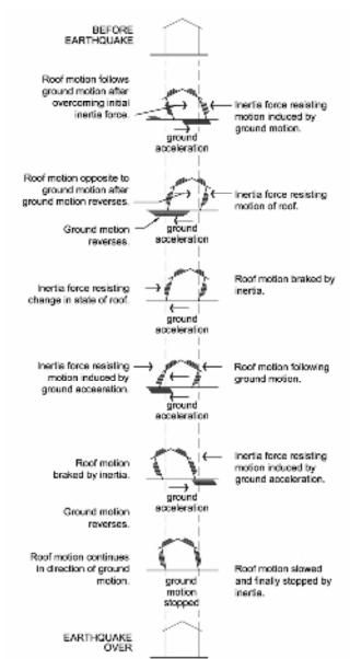
To perform adequately in an earthquake, a house must have enough strength to resist the forces generated without failure. Actual earthquakes can generate forces considerably higher than those used for code-prescribed design (Figure 1-3). Nevertheless, design for the lower code forces generally has prevented life loss and therefore satisfies the purpose of the code. Remember that
