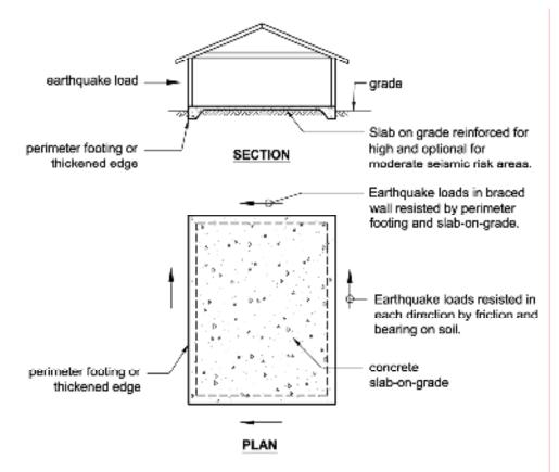
Figure 4-2 Slab-on-grade and perimeter footing transfer loads into soil.
