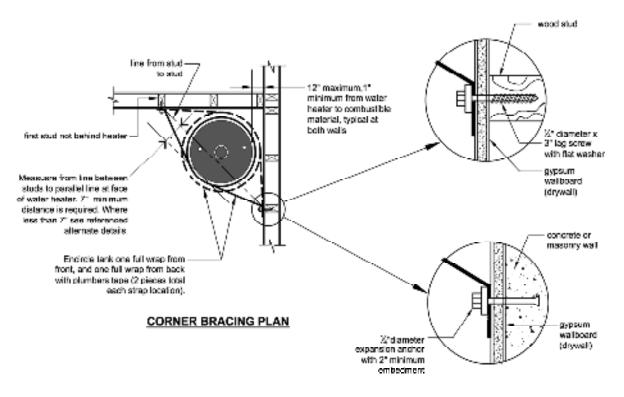
Figure 8-2a and 8-2b Securing a water heater with corner bracing.
