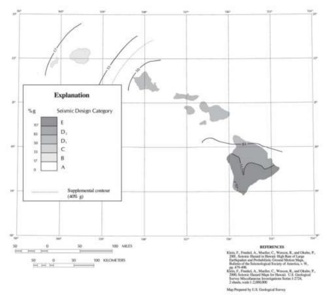
Figure 1-1 Seismic Design Categories – Site Class D (continued).
