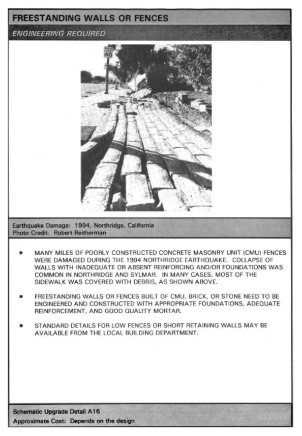
Figure 8-3d Reproduction of FEMA 74 suggestions for securing freestanding walls or fences.
