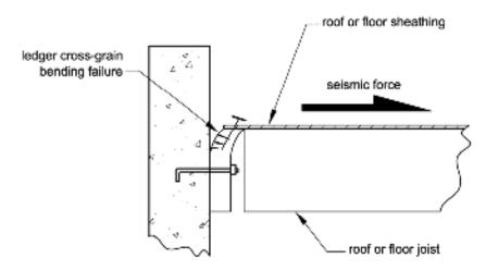
Figure 5-17 Illustration of cross-grain bending of wood ledger.
