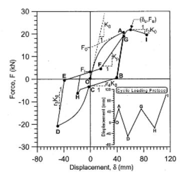
Figure A-6 Hysteretic parameters for model ((Folz and Filiatrault, 2002).
