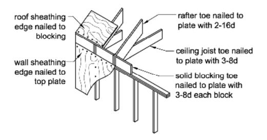
Figure 6-4 Blocking at rafters to exterior wall.
