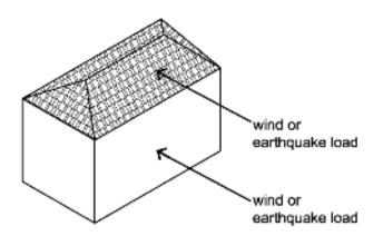
Figure 2-2 Lateral loads induced in a building due to wind or earthquakes.
