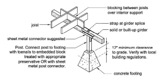
Figure 4-5 Interior bearing line.
