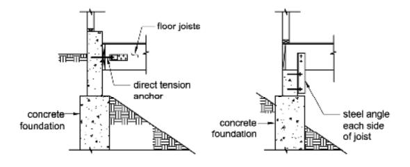
Figure 9-11 Anchorage of floor framing to the uphill foundation.
