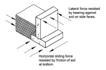
Figure 3-10 Lateral resistance provided by foundation.
