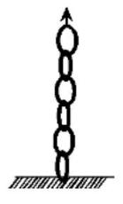
Figure 2-1 Chain illustrating the load path concept.
