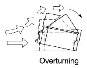
Figure 3-3 Overturning action resisted by foundation.
