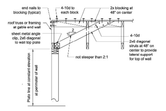
Figure 6-3 Gable end wall or gable truss bracing.
