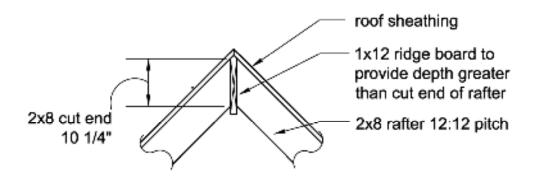
Figure 6-2 Ridge board for 12:12 pitch roof.
