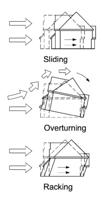
Figure 5-1 Sliding, overturning, and racking action resisted by walls and foundation.
