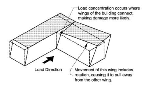
Figure 2-11 Concentration of loads and possible damage and failure due to irregular plan.
