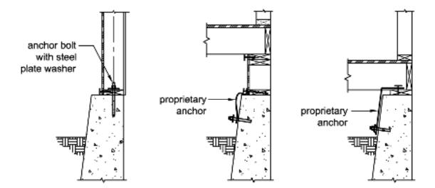
Figure 9-4 Common anchorage configurations.
