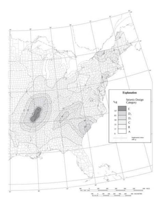
Figure 1-1 Seismic Design Categories – Site Class D (continued).
