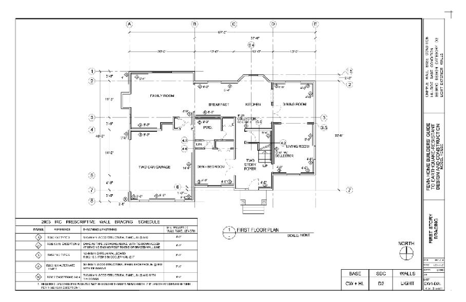
Figure 5-7b Plan view of first floor for model house with light-weight finish material located in SDC D<sub>2</sub>.
