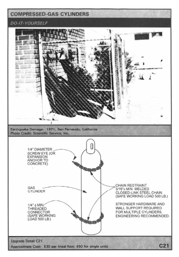
Figure 8-3e Reproduction of FEMA 74 suggestions for securing compressed-gas cylinders.
