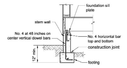
Figure 3-6 Recommended minimum reinforcement for concrete footings and stem walls.
