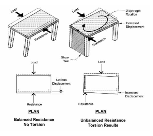
Figure 2-10 Rotational response and resistance to torsion.
