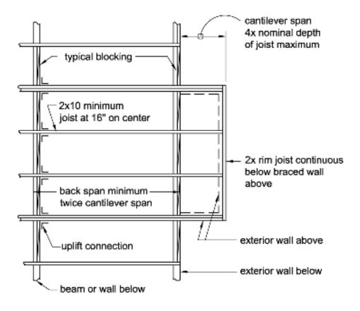
Figure 4-4 Cantilever joist at braced wall above.
