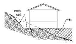
Figure 3-12 Foundation supported on rock and fill.
