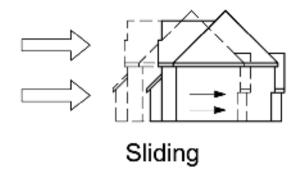
Figure 3-2 Sliding action resisted by foundation.
