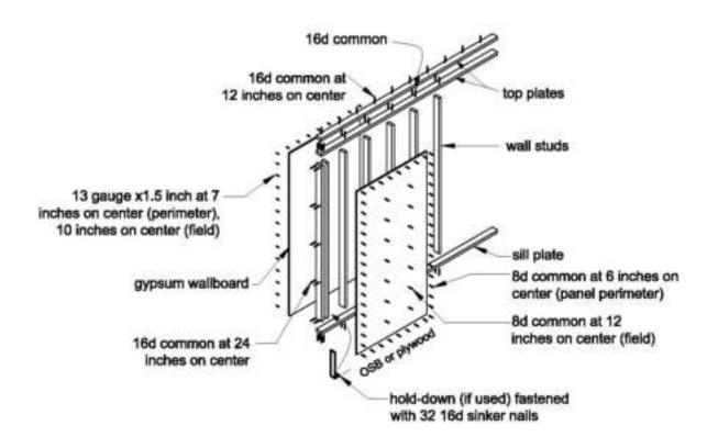
Figure 5-4 Exploded view of typical residential wall segment.
